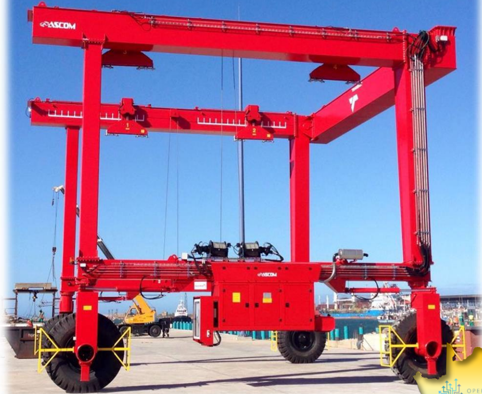
NEW 90 TON BOAT HOIST
